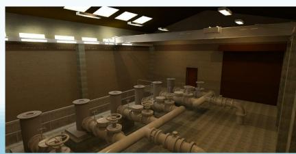
3-D BIM of interior of proposed Kent Pump Station Replacement.
