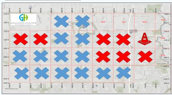
Above is the current 2019-2020 map of the valve inspections. The "X" indicates the area is complete, and the cone indicates the current location of inspections taking place. Blue indicates 2019, and Red indicates 2020 Year.
